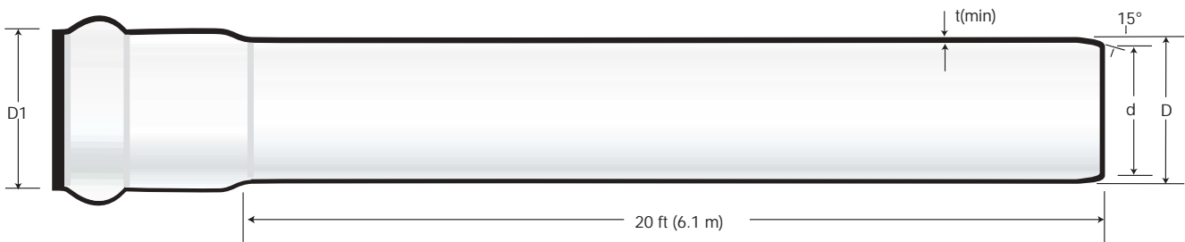
Fig. 2.3: AQUALOC Series gasketed bell pipe dimensions
