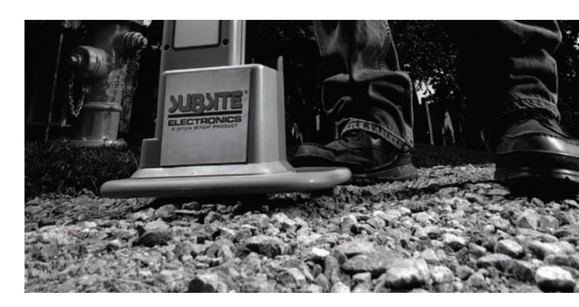
puried marker, and the marker returns a signal to the EML; location of the marker is indicated by an audible tone from the locator.
