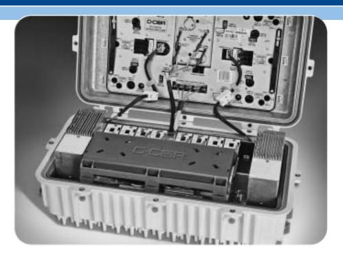
The Opti Max4100 1GHz Segmentable Node is C-COR's fully segmentable, modular, pay-as-you-grow node platform. The Opti Max4100 facilitates full 4 x 4 forward and return segmentation with an industry-leading port-to-port isolation. 1GHz will enable broadband service providers to increase forward capacity for HDTV over previous program offerings, thereby allowing a typically 40% increase over current HDTV channels in a lineup.
