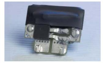
Constant - Repetitive AC RMS S4070 device......70 A Max. Voltage (Forward & Reverse) AC RMS. .400 V Max. Rate of "turn off" voltage ..1500 V/uSec. Rate of "commutation" voltage (dv/dt)... ..40 V/uSec. Voltage Triggering range (before activated)....140-170 V AC. Current (1 cycle) Non-Repetitive (60 Hz)..........950 A Max. Current (1 cycle) Non-Repetitive (50 Hz)...........800 A Max.
